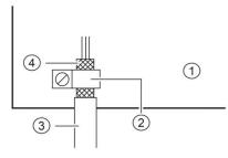
① mounting plate② conductive clamp③ data lines④ cable shielding
